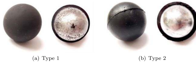
Fig. 1 Resonant inclusions used in the metaconcrete specimens. a Readily available commercial mouse balls. b Specifically manufactured rubber coated inclusions. Note that the type 2 inclusions present a circular interface due to the manufacturing process
