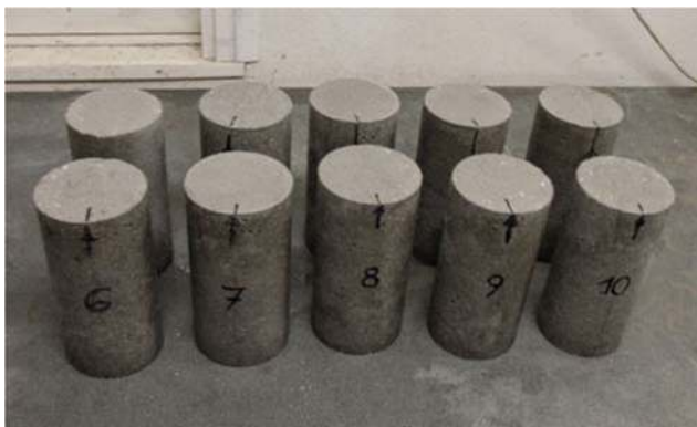
Fig. 6 Metaconcrete specimens after curing and final polishing.
