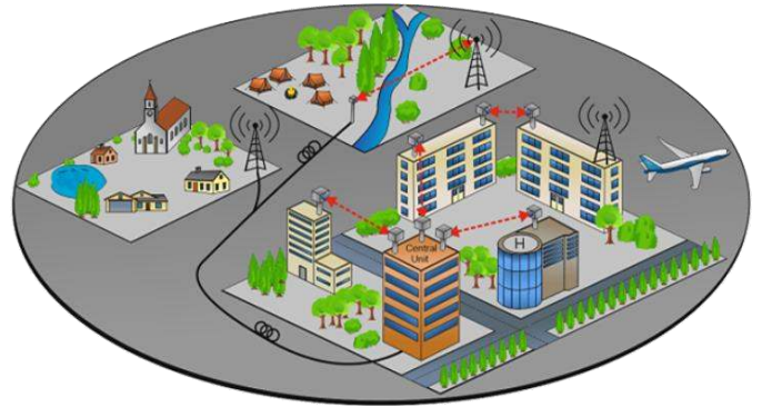
Fig. 1. Example of Radio over fibre and radio over FSO scenario adopting cloud RAN architecture.
