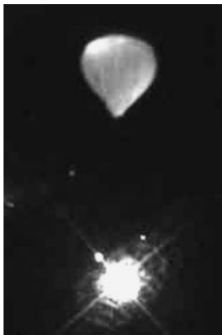
Figure 10. Near infrared picture of the stratospheric carrier with FELT from ground-station tracking camera after acquisition at approximately 60 km range.
