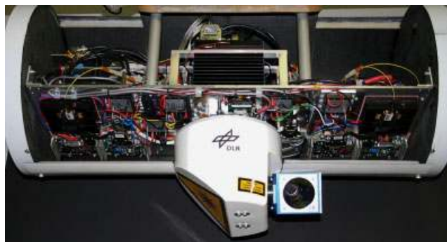
Figure 2. Assembly photo of FELT with opened housing.
