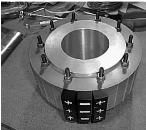
Fig. 14. Rotor magnets during the assembly process.
