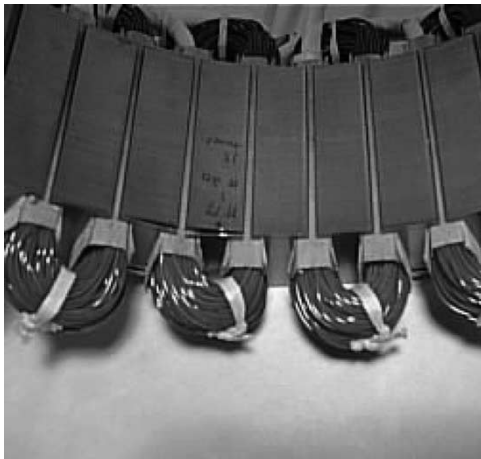
Fig. 13. Close-up view of concentrated winding with nonoverlapping end turns.
