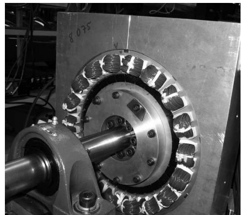
Fig. 17. End view of the machine after assembly, including bearings.
