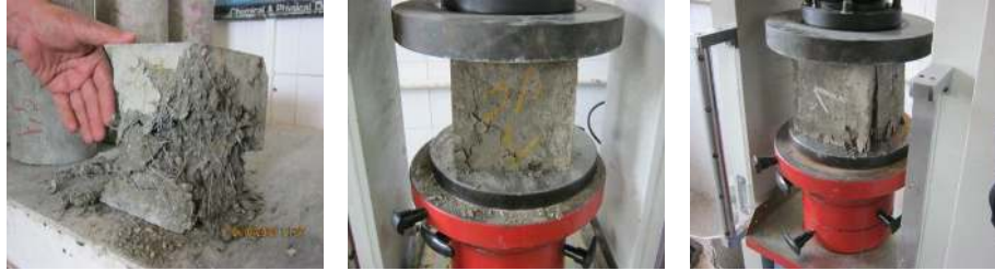
Figure 3 Images of compressive specimens containing steel fibres (see online version for colours)
