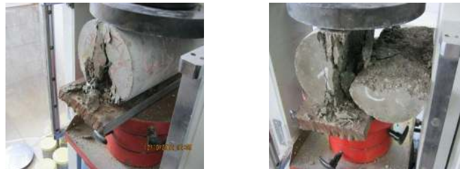
Figure 5 Images of cylindrical specimens with and without steel waste fibres (see online version for colours)
