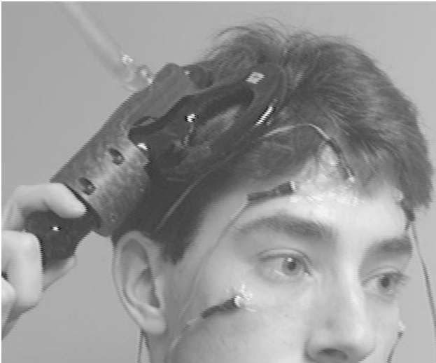
Figure 5. Subject set-up for TMS stimulation. LEDs mounted on the rod, orthogonal to the coil, track the position and orientation of the coil. LEDs taped to the face are used for tracking head motion.
