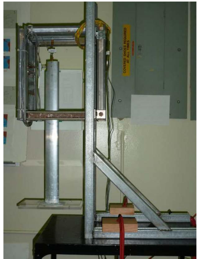
Fig. 2 The plate and strut are affixed to a rigid support structure that is positioned in the tank 2.62 m from the wavemaker and 5.22 m from the end of the tank
