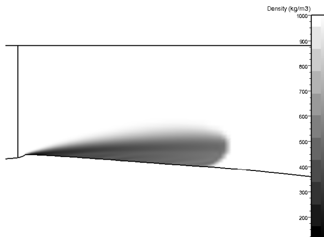
Figure N°20: Density field inside the cavity for A_{min}=50
