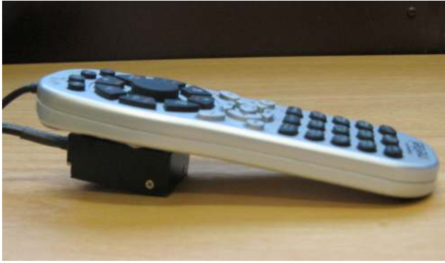
Figure 1. The mobile phone mockup device equipped with an Intersense Inertia Cube3 for motion tracking
