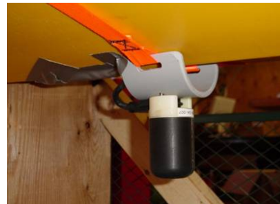
Fig. 3. Mounting of WHOI acoustic modem transducer on the Scout hull.
