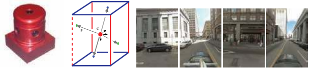
Figure 2. Panorama acquisition device. (a) Point Grey LadyBug camera. (b) A panoramic piecewise perspective image as an outer surface of the prism.
