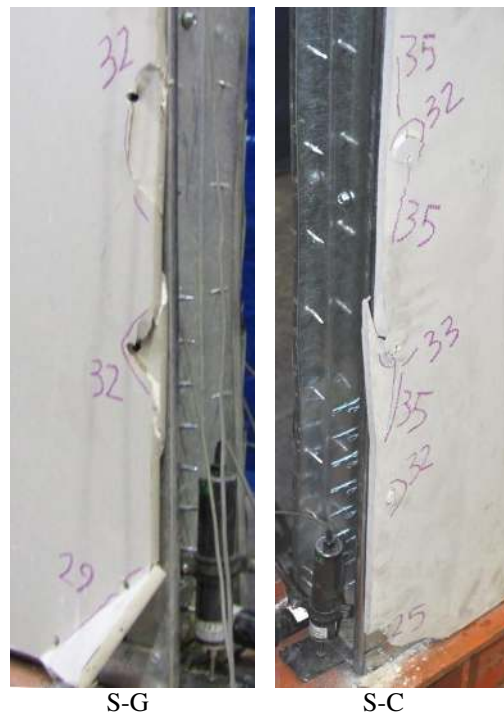
Fig. 10. Cladding fractures in region CD
