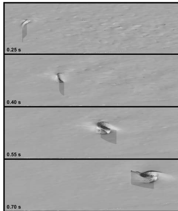
Fig. 7. Evolution of the free surface during the rowing stroke. Near the end of the stroke there is a surface bulge of approximately 10 cm above the blade and a depression of 8 cm behind the blade (Sliasis et al. [2009]).
