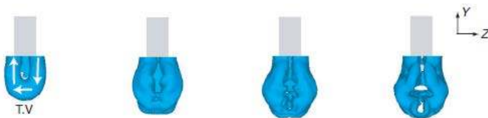
Fig. 11. Vortex formation process depicted using iso-surfaces of vorticity magnitude. The arrows in the first time step show the rotating direction of the vortex. T.V. indicates the position of the tip vortex (Gharib et al. [2011]).
