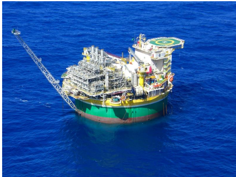
Figure 1. Sevan Piranema, the first Sevan circular-shaped FPSO.
