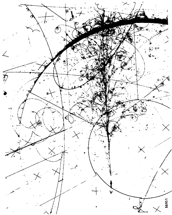
FIG. 3. A typical neutrino event as observed in the Big European Bubble Chamber (BEBC) filled with neon at the CERN 450-GeV Super Proton Synchrotron (SPS) accelerator. The muon can be seen on the left. It has been tagged by an external muon identifier. The many-particle hadron shower is to the right. Photograph by PHOTO CERN.
