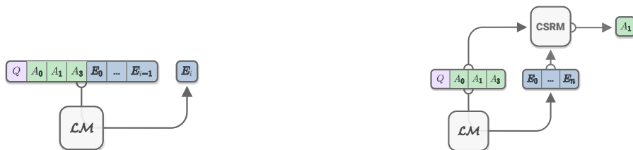
(a) One time-step of training a CAGE language model to generate explanations from CoS-E. It is conditioned on the question tokens Q concatenated with the answer choice tokens A_1, A_2, A_3 and previously generated tokens E_1, \dots, E_{i-1} . It is trained to generate token E_i . (b) A trained CAGE language model is used to generate explanations for a downstream commonsense reasoning model (CSR), which itself predicts one of the answer choices.
