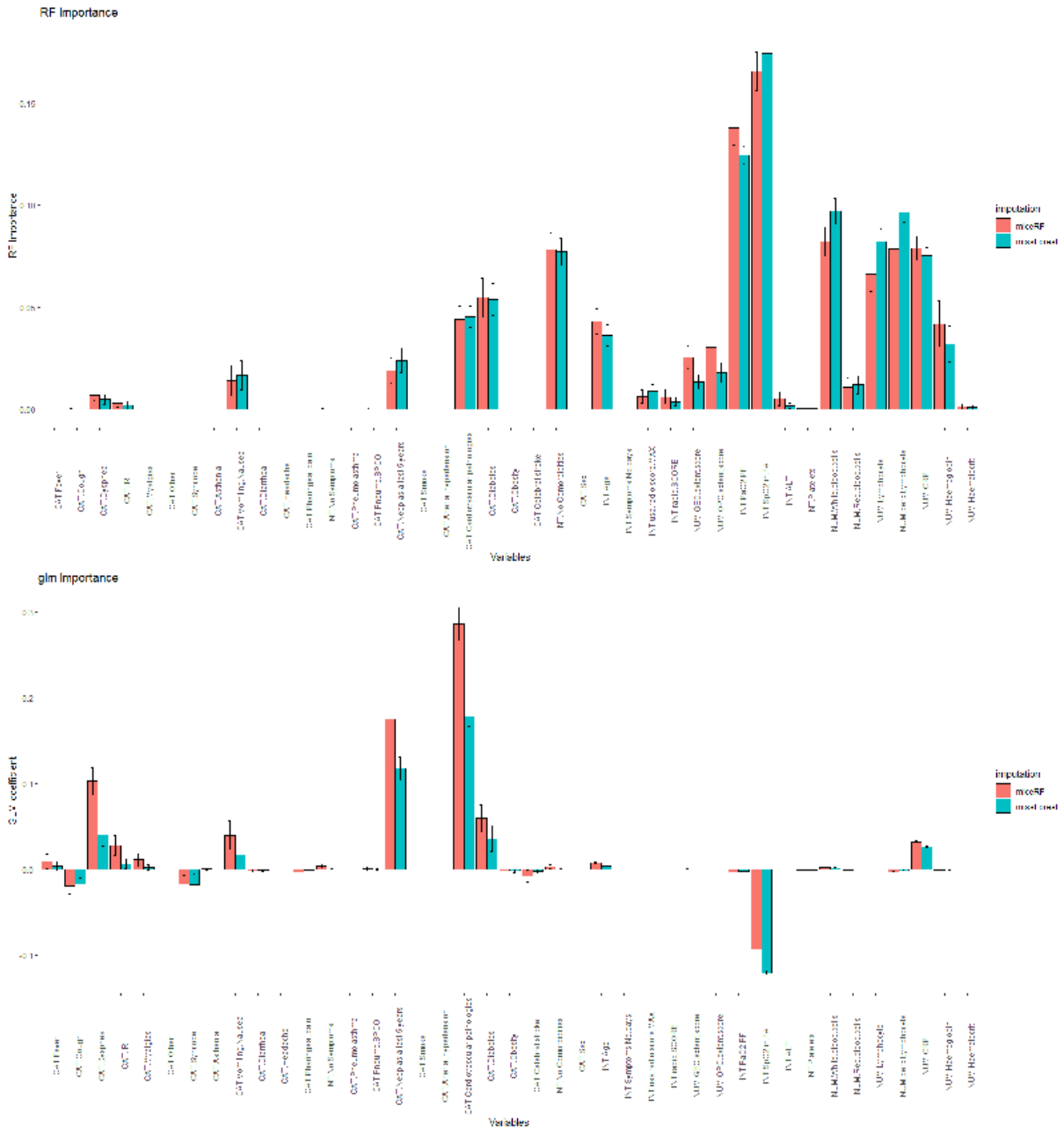
FIGURE 7. Top: estimates (and standard errors) of the feature relevance computed by RFs. Bottom: estimates (and standard errors) of the feature coefficients computed by GLMs. Only the significant feature relevances/coefficients are plotted.
