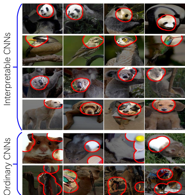
Fig. 15 Illustration of the interpretable CNN designed by Zhang et al. 118 . The top four rows show example filter feature maps from the interpretable CNN and the bottom two rows show example filter feature maps from an ordinary CNN. Note that feature maps from the interpretable CNN filters tend to be meaningful (animal heads in this example) while feature maps from ordinary CNN filters are usually meaningless. These filter feature maps are computed from filter receptive fields following a technique proposed by Zhou et al. 161 . Figure reprinted from ref. 118 with permission. Copyright 2018 IEEE.
