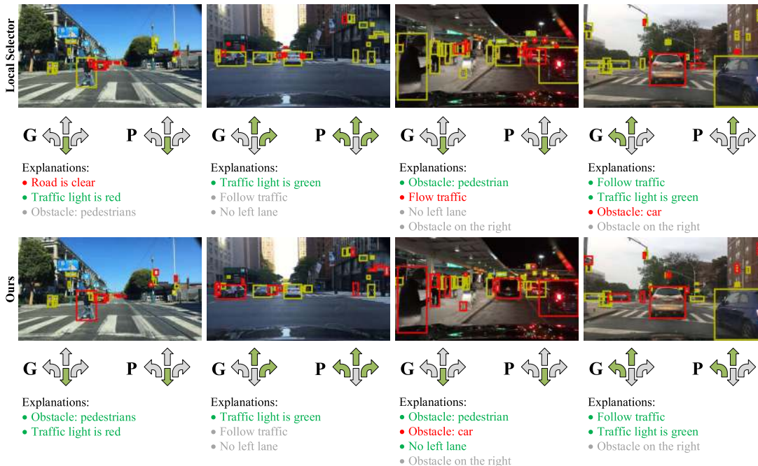
Figure 4. Examples of network predictions, objects selected as action-inducing, and explanations. Yellow bounding boxes identify the objects detected by the Faster R-CNN, while red bounding boxes identify the objects selected as action-inducing by the proposed network. “G” stands for ground truth and “P” for prediction. For explanations, green indicates true positives, red false positives, and gray false negatives ( i.e. valid explanations not predicted).
