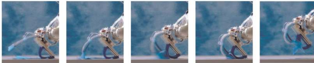
(b) Surface-constrained grasp picking up a piece of tissue, from left to right: exploitation of table to position and orient the hand, exploitation of table to ensure contact with the flat object, compliant grasping, established grasp, and object lift
