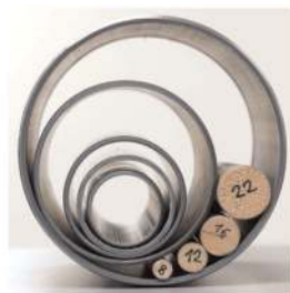
(a) Cylinders with 8, 12, 16, 22, 32, 40, 50, 75 and 110 mm diameter
