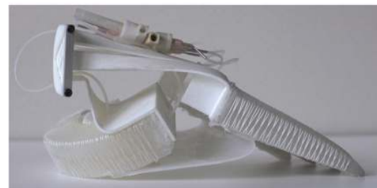
Fig. 15. RBO Hand 2 consists of a flexible polyamide scaffold on which four fingers and a palm–thumb compound are mounted. Fingers and palm are made of PneuFlex continuum actuators. On its backside splitters are attached to distribute air from two actuation channels to the individual actuators.
