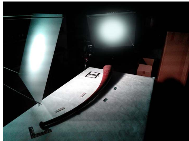
Figure 2: Multispectral photogrammetry setup used to digitize the horn.
