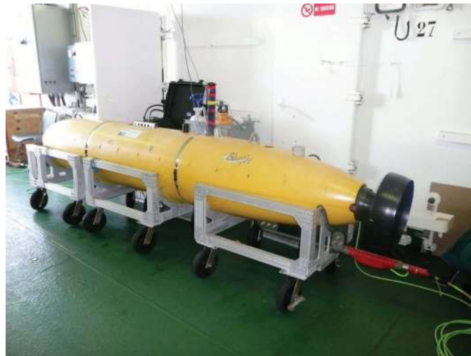
Fig. 2. The Bluefin 21" Unicorn AUV operated by the MIT Laboratory for Autonomous Marine Sensing Systems. Used with permission from [19].
