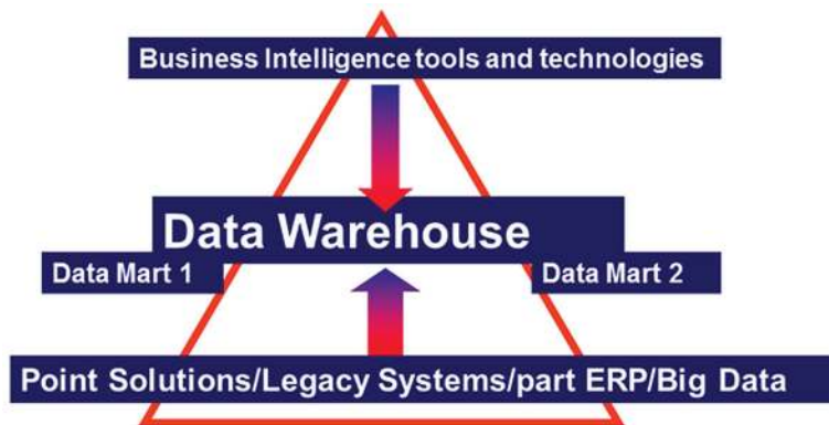
Figure 1. Typical systems architecture underpinning BI tools deployment
