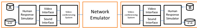
Figure 9: The architecture of RealTalk , an evaluation testbed for proprietary video conferencing systems.
