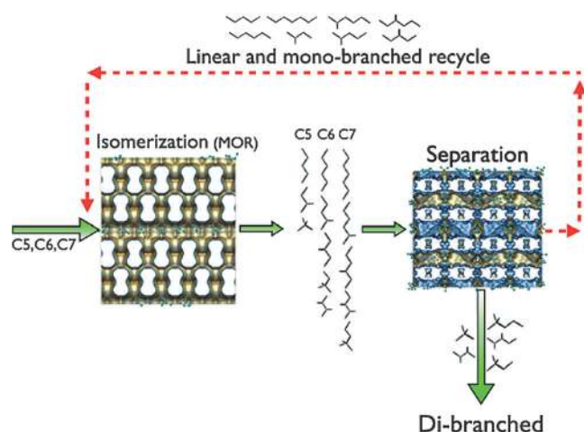
Figure 16. Schematic of the separation process. The feed consists of mostly linear alkanes. First, the linear alkanes are isomerized to branched alkanes (usually using MOF-zeolite). Next, the linear and mono-branched alkanes are separated from the desired di-branched alkanes and recycled back.
