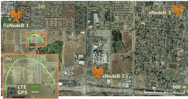
Fig. 18. (a) Environment layout, eNodeBs' locations, and the traversed trajectory. (b) The receiver's GPS trajectory estimate and the trajectory estimated using LTE signals. The RMSE between the GPS and LTE navigation solutions was calculated to be 8.15 m with an estimation error standard deviation of 2.83 m and a maximum error of 12.38 m. Image: Google Earth
