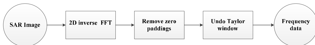
Figure 7. Procedure of transforming SAR images to the frequency domain. 2D: two-dimensional; FFT: fast Fourier transform.
