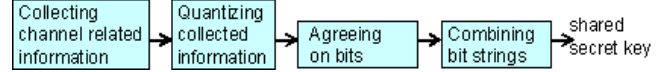
Fig. 2. Steps of generating shared secret keys in multiple-antenna systems using the channel related information.
