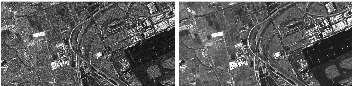
Fig. 2. Single-look TerraSAR-X image of Barcelona (image courtesy ©Infoterra GmbH) and the radiometry estimated by the nonlocal method [11]. Images are 511 \times 1043 pixels with a spatial resolution of 2.5 m.
