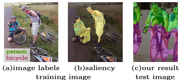
Figure 1: We train a semantic labelling network with (a) image-level labels and (b) saliency masks, to generate (c) a pixel-wise labelling of object classes at test time.
