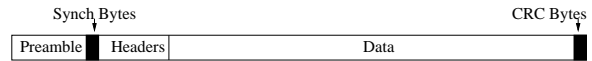
(a) PacketFormat A packet contains a preamble, a synchronization byte, the packet headers, the data and CRC bytes.
