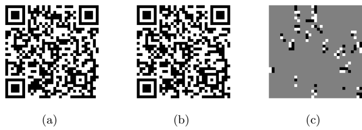
Fig. 4. Secret and reconstructed secret for the example shown in Fig 3. (a) Original QR code containing the secret message, S . (b) Reconstructed secret QR code, S^r . (c) Difference image between S and S^r .
