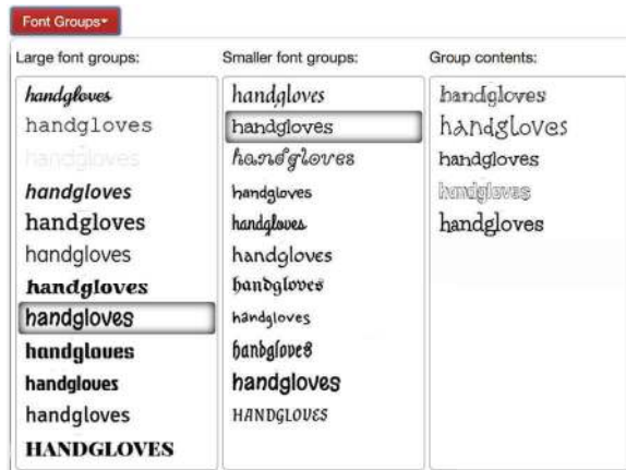
Figure 2: Group interface. The interface shows a three-level perceptual clustering of fonts. Mousing over the clusters allows a user to quickly get a sense of the range of options, and to explore individual clusters. Once a user has selected a font, they may further refine their query by searching for similar fonts as in Figure 1.
