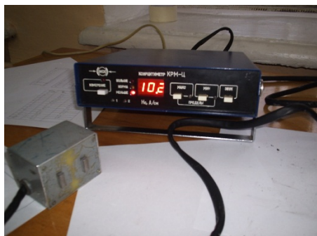
Fig. 2. General view of coercimeter KRM-C (Russia)
