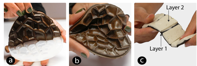
Figure 11: a. Demolding the biofoam sample. b. Biofoam acts like memory foam, c. Biofoam applied in layers.
