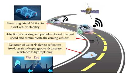
**Figure 14.** Potential benefits from vehicle mobility patterns with connected tires (adapted by [98]), case of an interurban road environment.
