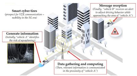
Figure 13. The concept of cyber smart tires (adapted by [95]), case of an urban road environment.
