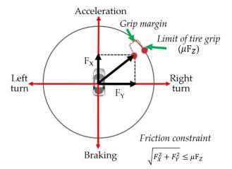
Figure 2. Friction circle during vehicle typical maneuvering [32].
