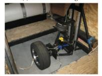
(d) Mobile tire test rig attached to the towing vehicle
