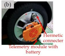
**Figure 12.** Example of an intelligent tire system setup and its installation parts: (**a**) accelerometer and (**b**) additional equipment components [86].
