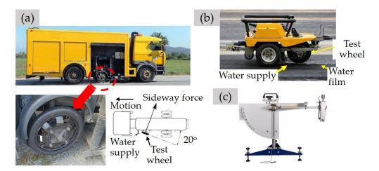
**Figure 7.** Typical systems for skid resistance measurements: (a) SCRIM system, (b) GripTester system (trailer-towed) and (c) a portable BPT system.
