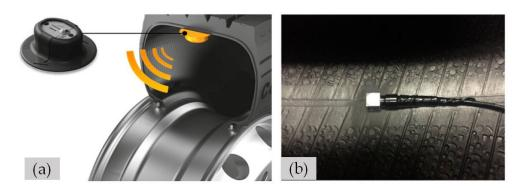
**Figure 9.** Typical examples of (a) adhesive tire sensors and (b) adhesive tread sensors (tri-axial accelerometer).
