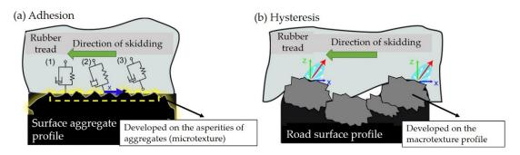
Figure 5. Illustration of (a) adhesion mechanism and (b) hysteresis mechanism (adapted from [45]).
