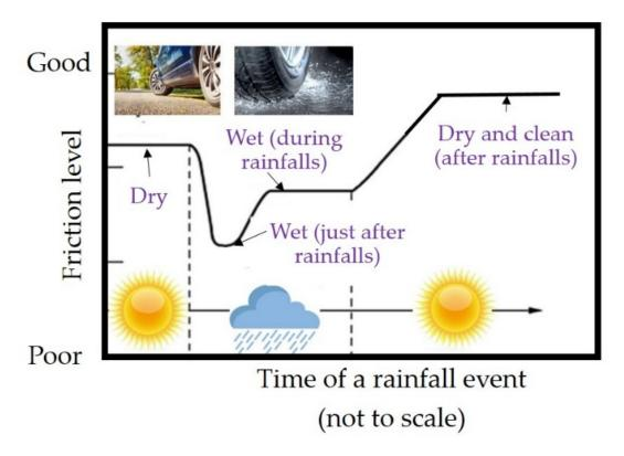
**Figure 6.** Friction level variations of a pavement surface subject to weather changes (adapted from [55]).
