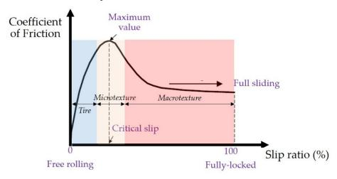
Figure 3. Friction versus tire slip (adapted from [33]).
