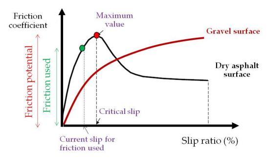
Figure 10. Friction versus longitudinal slip for differently paved surfaces (adapted from [45]).
