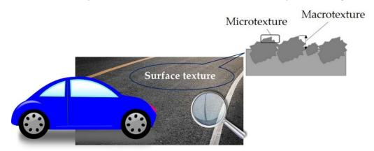
Figure 4. Illustration of pavement texture components.
