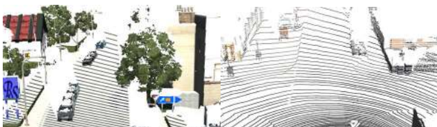
Figure 5: We train our network on synthetic point clouds generated from vKITTI [8] (left) and apply it onto real-world Velodyne LiDAR point clouds (right). The structure and the varying density are comparable.
