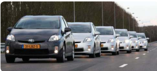
FIGURE 2 A platoon of vehicles that cooperatively regulates the intervehicle spacing to improve traffic flow. Wireless communication is used to transmit acceleration setpoints between adjacent vehicles. (Image courtesy of NWO, The Netherlands.)
