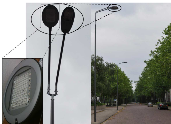
Fig. 5. LED and HID luminaries (left), a view from the testbed (right).
