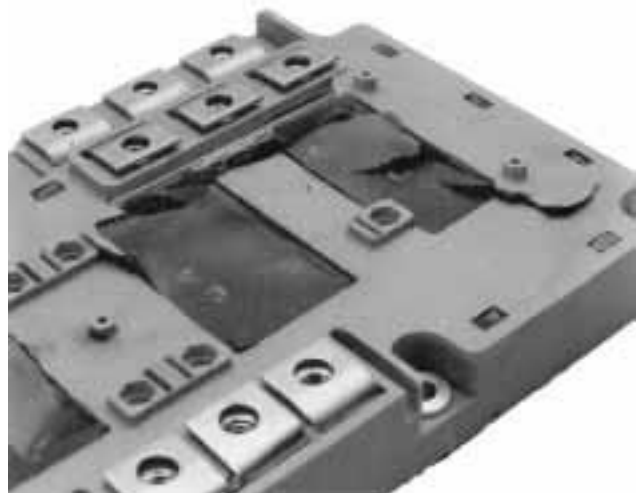
Fig.4 Discharge of 10 kJ into a phase-leg module (Test A). This module contains the high and low-side in one package.
