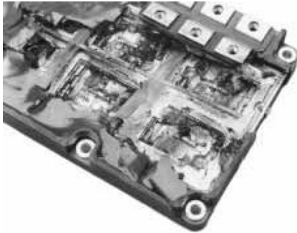
Fig. 5 LS module after a discharge of 20.3 kJ (Test B). Massive ejection of gel and rubber particles occurs. The terminals are bent, but still in place.
