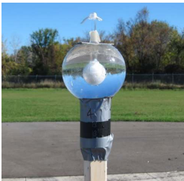
Fig. 2 Photograph of a 1 L glass sphere containing distilled water. Central burster contains 28 g C4
