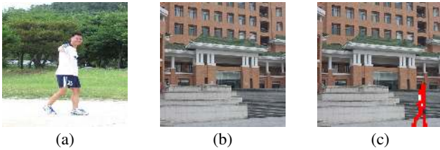
Fig. 4. Cut-and-paste forgery detection example using 64 \times 64 pixels blocks. (a) The original image from which an object is cut, (b) the original image onto which the cut object is pasted, (c) the detection result.
