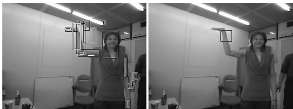
Fig. 4 Marked regions of interest. Black and white rectangular regions denote skin and motion area, respectively. A black rectangular region in the right snapshot denotes the average position of the fastest moving skin color objects. Tracking of multiple objects is possible because of the parallel processing framework
