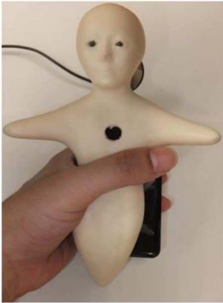
FIGURE 1 | Elfoïd: cellular phone-type teleoperated android.
