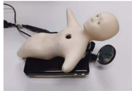
FIGURE 2 | Elfoïd with a mobile projector to convey the facial expressions of a communication partner.
