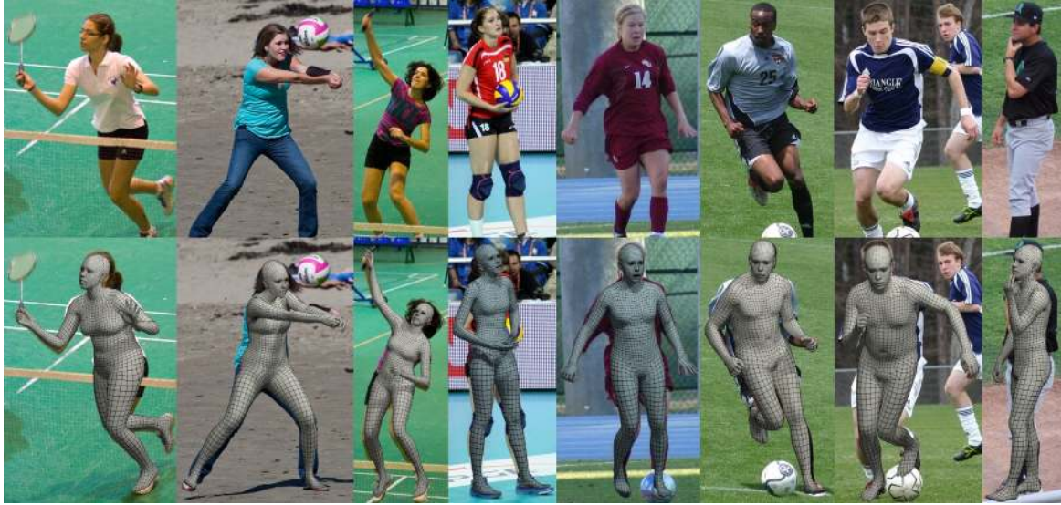
Figure 4: Qualitative results of SMPL-X for the in-the-wild images of the LSP dataset [33]. A strong holistic model like SMPL-X results in natural and expressive reconstruction of bodies, hands and faces. Gray color depicts the gender-specific model for confident gender detections. Blue is the gender-neutral model that is used when the gender classifier is uncertain.
