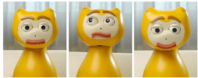
Figure 1. iCat: Robotic research platform for human-machine interaction developed by Philips Research
