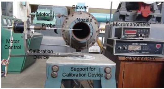
FIGURE 2: Calibration tunnel, calibration device, probe, and instrumentation.
