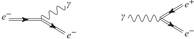
FIG. 3. Feynman diagrams for the two basic processes included in the PIC approach. Time flows from left to right. A straight line indicates an electron or positron interacting with an external field (e.g. an intense laser), and a wavy line is a photon. Left : nonlinear Compton scattering. Right : stimulated pair production.
