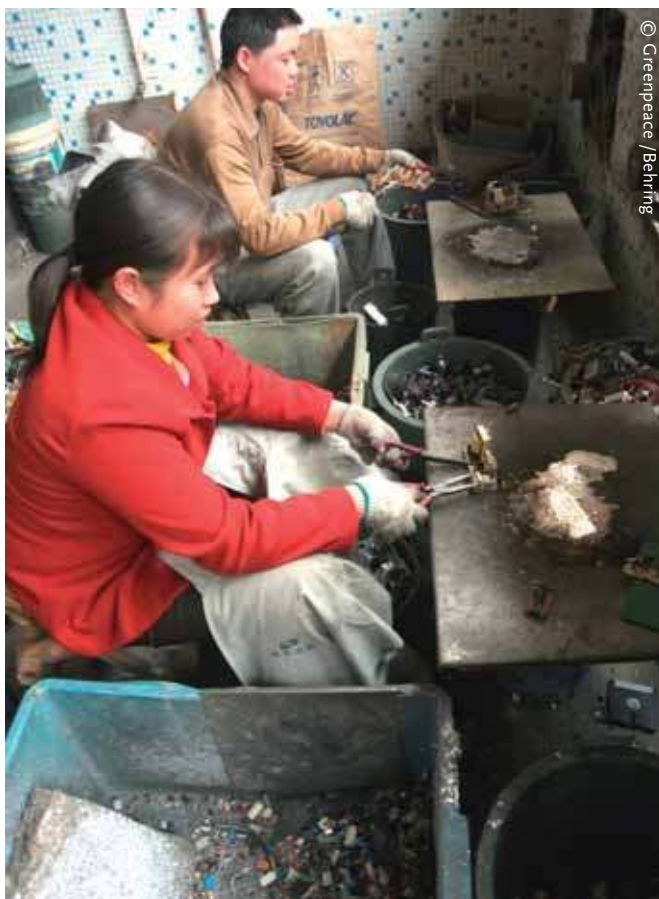
Women workers 'bake' motherboards from e-waste, breathing toxic fumes, in Nanyang, China.
