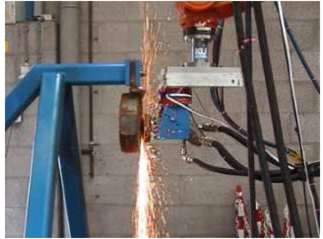
Figure 5: Grinding with IRB6400 at Kranendonk, the Netherlands, using a compliant grinding tool developed at KU Leuven, Belgium, together with force feedback control. The video can be found at www.robot.lth.se .
